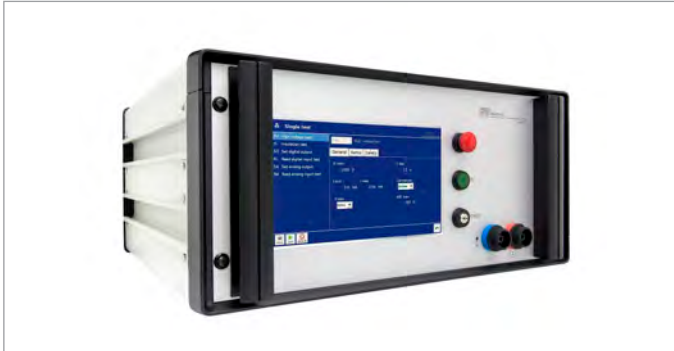
Hipot test device HA 1885G / HA 1885J Plug-in 19" / 5 HU in housing
